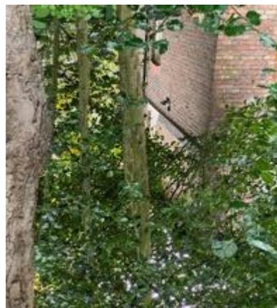
Opposite is a photo of the trees against the Old Rectory. This is an example of the numerous trees that have grown very close to or against buildings. This has two affects; the first is the transference of damp into the brick work and the second the clogging up of the gutters and drains with leaves. The roofers, who have nearly finished the remedial work at Our Lady's, have spent time clearing the gutters and drainpipes
